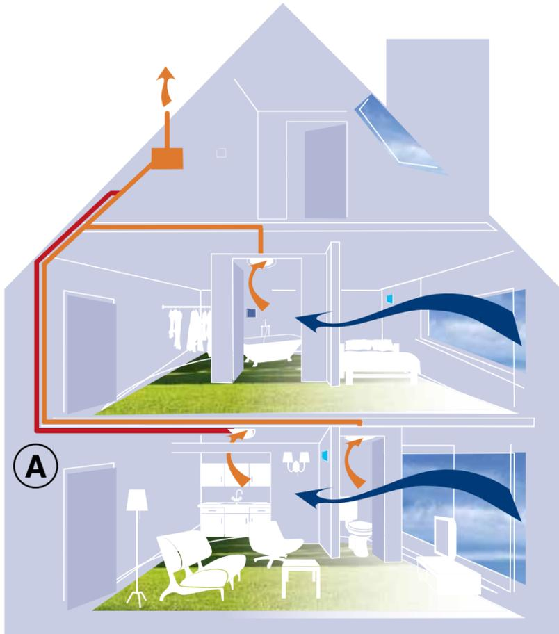
**Fig A** - Illustrates a typical "System 3" or central extract duct layout, focusing on the 'Best Practice' that the toilet extract is separate to, or positioned in line between the kitchen extract and the extract unit.
